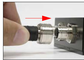
Microscan QX-830 with M12 Ultra-Lock Connector
