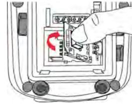
4. Insert the SIM card into the cover with notched corner up, and the contact side of SIM card faces down.
