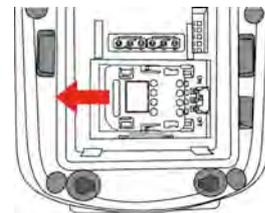
6. Put the battery back into the battery compartment and replace the battery compartment cover.
