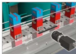
Simultaneous reading of barcodes and characters
