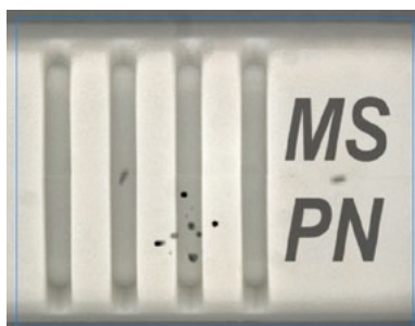
Minute flaw detection exist on the background having printed characters and surface irregularities.
